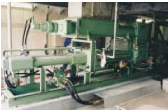
The El Indio gold mine backfill pump transports a 76% Cw cement based paste fill to the voids left by the mining operations. The paste mixer discharges into the hopper, which is open and tapered to suit the feed requirements. South Deep mine in South Africa transports backfill over 1250 metres from the underground crushing plant to the elevated stopes where the 85% Cw mixture of crushed waste and 15 mm aggregate helps to prevent rock bursts.
