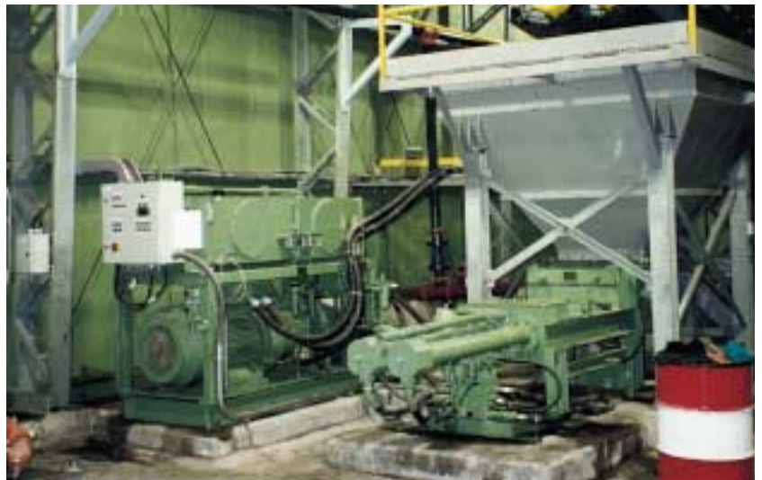
The El Indio gold mine backfill pump transports a 76% Cw cement based paste fill to the voids left by the mining operations. The paste mixer discharges into the hopper, which is open and tapered to suit the feed requirements. South Deep mine in South Africa transports backfill over 1250 metres from the underground crushing plant to the elevated stopes where the 85% Cw mixture of crushed waste and 15 mm aggregate helps to prevent rock bursts.
